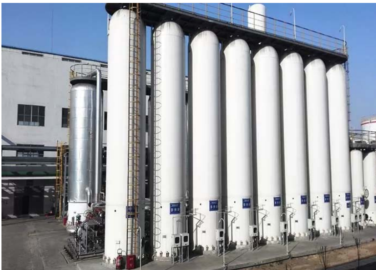
Figure 6: Multiple pressure swing adsorption (PSA) columns for hydrogen purification. Vacuum PSA or temperature swing adsorption, which are related to the purification process, can also be used for carbon capture. Process CO 2 only accounts for 60 – 70% of the overall CO 2 emissions, the remainder being related to energy requirements for the process.
